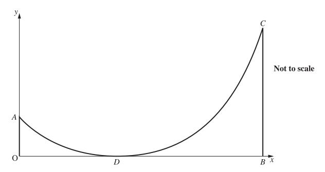
It is required to find the height of pole BC by modelling the shape of the curve that the chain forms.
